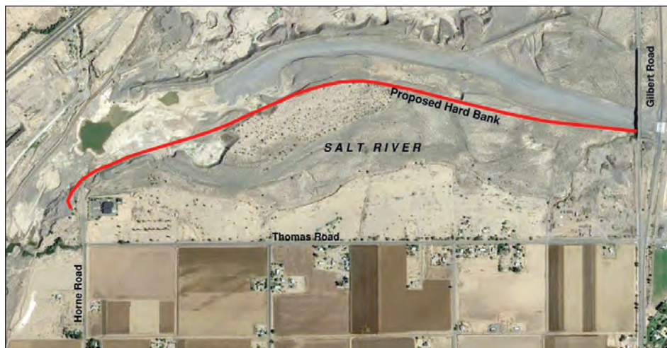
The ECS staff is working on the Hard Bank Project, which will mitigate erosion on the south bank of the Salt River from the Gilbert Road Bridge to Mesa Drive. The hard bank will restore any erosion of the riverbank by protecting it with soil cement. These two images show where the areas will be restored and how the hard bank will protect Lehi from an overflowing Salt River when water is released from the Granite Reef Dam. Photos courtesy of ECS Construction Managers Steven Pokrzywka
