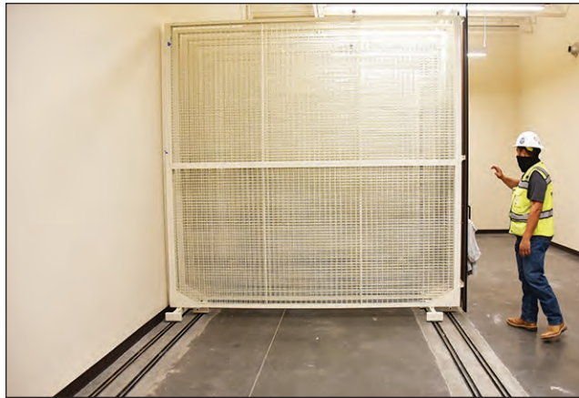
Shelves for artifacts on rails that can move back and forth, from the OAN tour on March 25.
