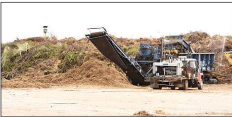
Dirt and plant matter being set aside from the other waste that comes through the Salt River Landfill.
